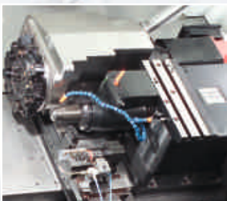
Turret and sub spindle
